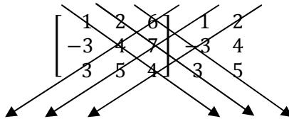
$$(\vec{u}, \vec{v}, \vec{w}) = \left[ \underbrace{1.4.4}_{16} + \underbrace{2.7.3}_{42} + \underbrace{6.(-3).5}_{-90} \right] - \left[ \underbrace{6.4.3}_{72} + \underbrace{1.7.5}_{35} + \underbrace{2.(-3).4}_{-24} \right]$$
